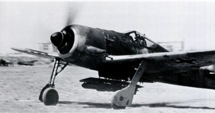
Above: A taxiing Fw 190 equipped with an ER 4 rack which allowed four bombs each of 50 kg to be carried. The weapons seen here appear to be SC 50s.
