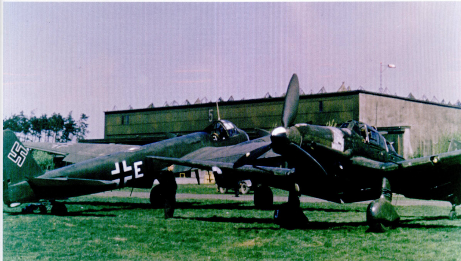
Two photographs of Ju 87D-5 W.Nr. 140736, V8+JB of 1./NSG 1, after its capture along with other Luftwaffe aircraft at Wunsdorf aerodrome on 7 April 1945 by the British 5th Parachute Brigade. Of note are the absence of dive brakes, a white "J" on the starboard wheel spat and a Balkenkreuz under the wing. The aircraft appears to have suffered a localised fire to the rear of the engine on the starboard side (below) with just scorching to the port cowling in the above photo. In the background is a Junkers Ju 88A-4 F1+EU of III./Erg. KG 1.
