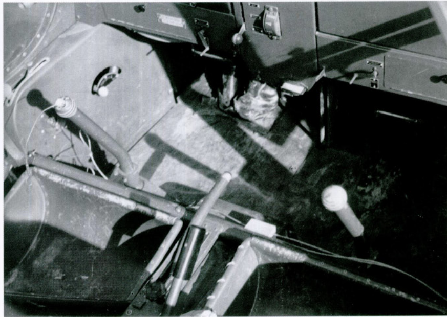
A view into the cockpit of the defected Bücker showing the simple trigger cabling for the four wing-mounted Panzerfaust. The observer who sat in the right-hand seat fired all four at once by simply pulling on this cable.
