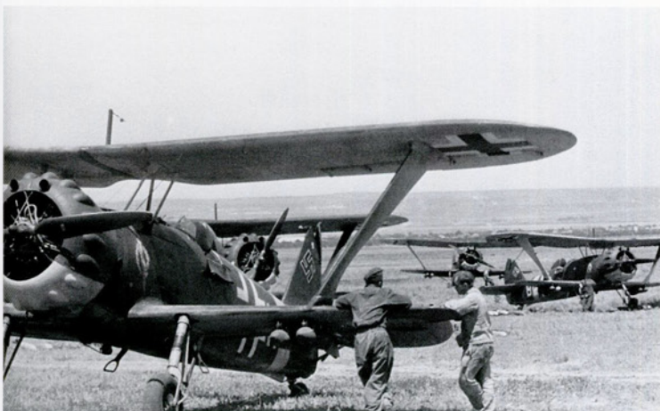
The Hs 123 was frequently able to continue operations when airfield conditions had grounded other types, operations from soft forward airstrips being facilitated by the removal of the undercarriage fairings, as shown on these machines of 7./Sch.G 1 photographed in Russia in 1942. Note the SC 50 bombs under the wings and the Infanteriesturmabzeichen stencilled on the forward fuselage. Although the Infantry Assault Badge became especially popular as an aircraft marking during the Russian campaign, it had earlier been used on the Hs 123s of II.(Schlacht)/LG 2 in Greece.
