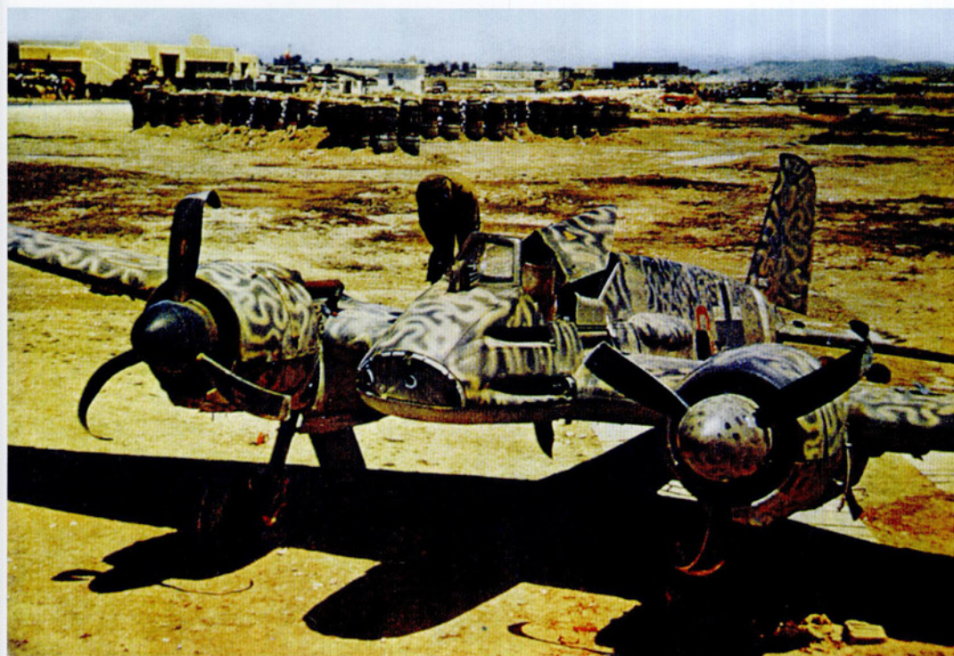
This Hs 129 B-2 'Red C' of 8.(Pz)/Sch.G 2 was found by the British at El Aounia, Tunisia in early 1943. The camouflage on this aircraft consisted of an almost continuous wavy line sprayed in a sand colour over the standard splinter pattern RLM 70/71 green, with the under surfaces in RLM 65 light blue. The aircraft had evidently suffered a wheels-up landing with the engines still turning, but had since been raised and then had the undercarriage lowered.
