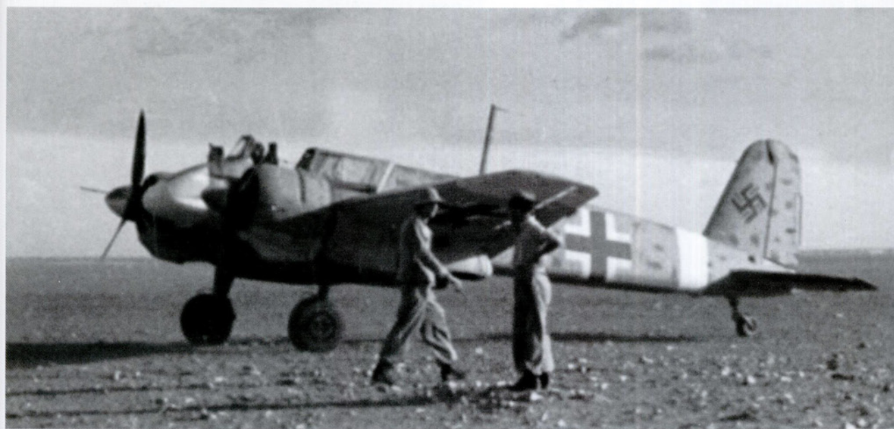
This Hs 129 B-2 'Red C' of 8.(Pz)/Sch.G 2 was found by the British at El Aounia, Tunisia in early 1943. The camouflage on this aircraft consisted of an almost continuous wavy line sprayed in a sand colour over the standard splinter pattern RLM 70/71 green, with the under surfaces in RLM 65 light blue. The aircraft had evidently suffered a wheels-up landing with the engines still turning, but had since been raised and then had the undercarriage lowered.
