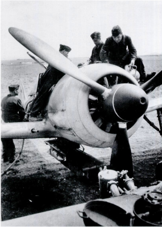
Luftwaffe ground personnel arming and refuelling a ground-attack Fw 190. Note the 'Ironing Board', the Luftwaffe's name for the ER 4 rack mounted under the fuselage.
