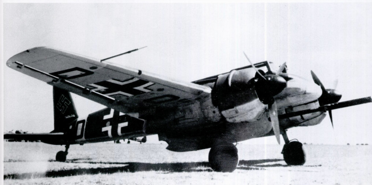
The concept of the 75 mm airborne anti-tank cannon was later taken up by the Henschel factory in Berlin and installed in a specially converted Hs 129 B-2, W.Nr. 140494, shown here. This proved more successful than the earlier Ju 88 P-1 and the type eventually went into production on a small-scale as the Hs 129 B-3.
