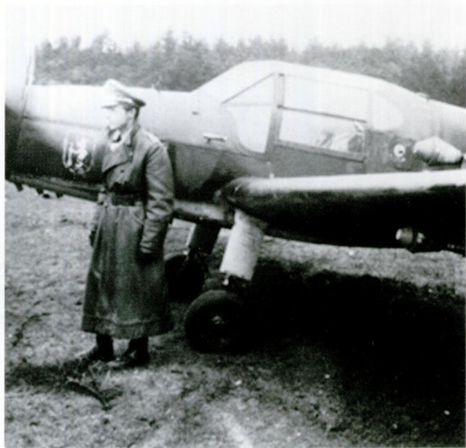
Above and below: Two views of either side of a Bü 181 of 1. Tiefangriffsgruppe Buecker 181 photographed in March or April 1945. Both views show single Panzerfaust fitted to racks mounted on to the upper and lower surfaces of each wing. The photograph above shows Oblt. Loesener; note also the crude site arrangement on top of the cowling. The photograph to the left shows a pilot NCO in a flight suit, Ofw. Paetzsch.
