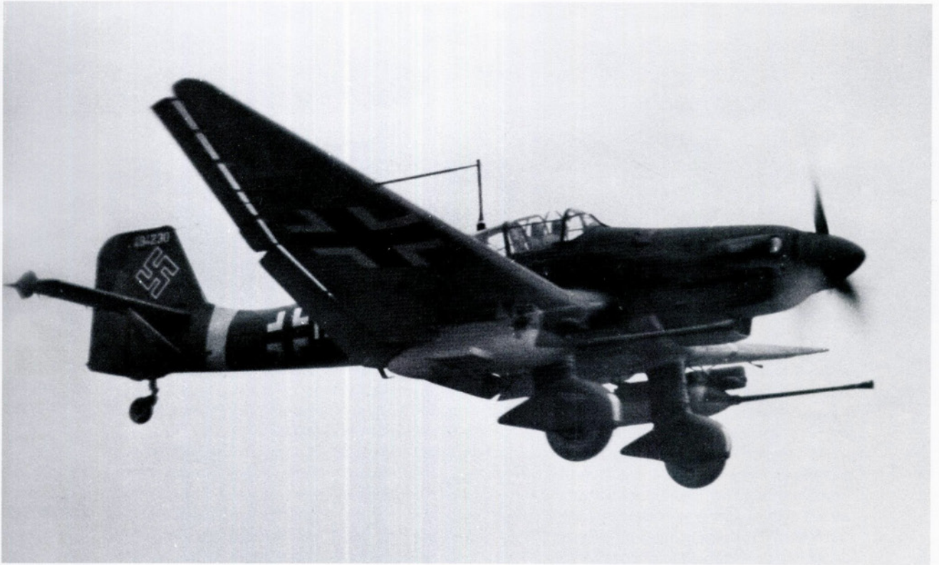
In this view of a Ju 87 G-2 armed with two 37 mm anti-tank cannon, it may be appreciated why Soviet fighter controllers referred to such machines as "the Stuka with the two long bars". This particular aircraft, W.Nr. 494230, flew with 10.(Pz)/SG 2 and was coded T6+MU with the unit code in smaller characters. The individual aircraft letter 'M' was in white, the Staffel colour, and was repeated on the front of each wheel fairing.
