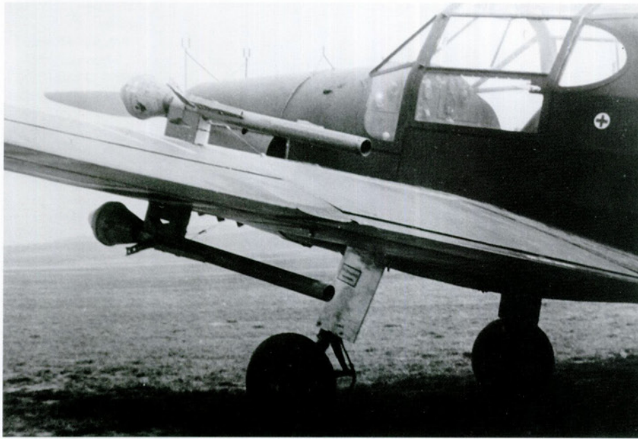
A Bücker Bü 181 fitted with two wing-mounted Panzerfaust 100m anti-tank missiles. The Panzerfaust were positioned in a five-degree nose-up attitude and launched from makeshift racks fitted at a central point on the wing. It is believed that some 150-170 Bü 181 trainers were converted to such a configuration.
