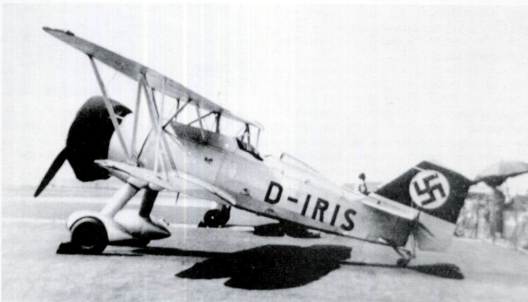
Two Curtiss F11C-2 Hawk dive bombers were bought by the German Defence Ministry following a visit by Ernst Udet to the USA in 1931. After extensive testing these were presented to Ernst Udet for his personal use. These aircraft were to stimulate the Luftwaffe 's interest in the dive bomber.
