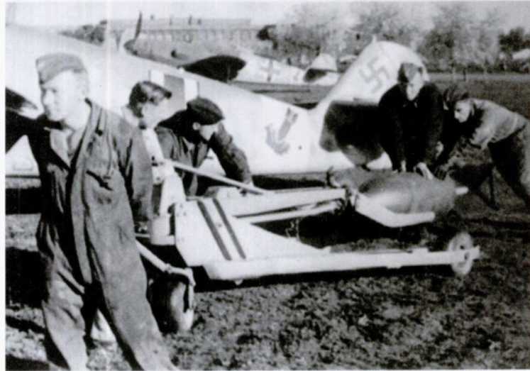
Ground crew push a hydraulic bomb trolley loaded with a SC 250 bomb past a Bf 109 F of 10.( Jabo )/JG 53.
