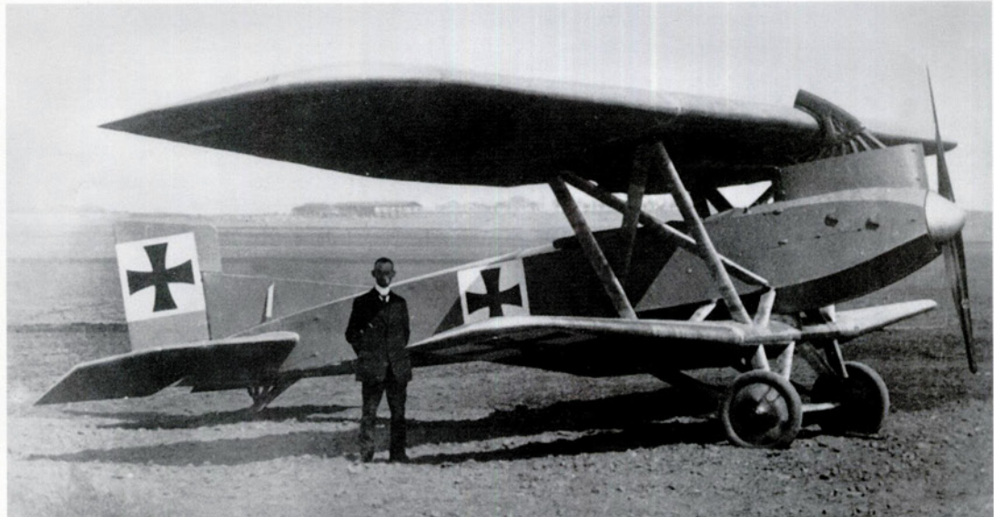
The Junkers J.I was the first aircraft in the world designed for the role of specialised close-support. It was a two-seater built of metal and featured a 5 mm armoured nose section which protected both engine and crew. The type entered service towards the end of 1917 and its strong construction proved extremely popular with its crews.
