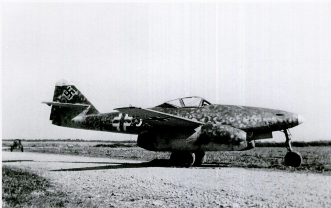
An Me 262 A-2a fighter-bomber photographed just after delivery to I./KG 51. Coded 9K+YH, the aircraft had sprayed "scribble" pattern camouflage with white fuselage nose tone, fin and rudder tip and individual letter. This aircraft has only two gun ports for its MK 108 cannon, but others, while carrying a similar armament, still had all four ports visible.
