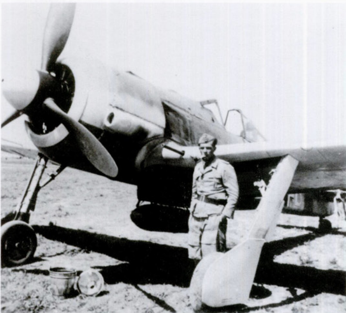
Another unidentified Fw 190 in North Africa, this example having external sand guards fitted to the air filter. On untropicalised aircraft, the air filters were concealed under blisters on the engine cowling.
